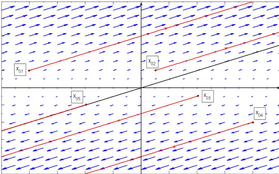
Fig. 4.1.12 - Vector field diagram for distinct real eigenvalues: one null, the other positive.
