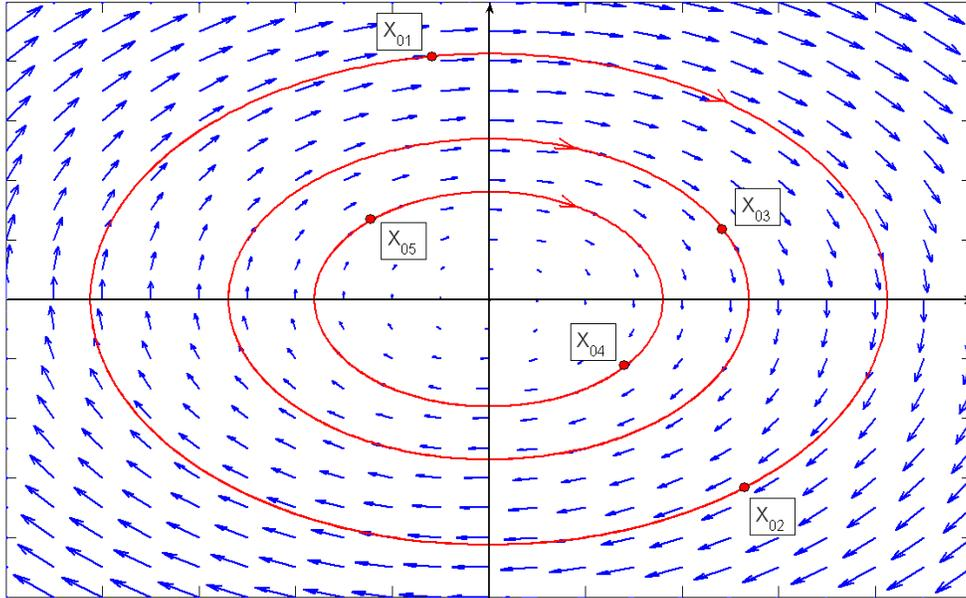
Fig. 4.1.6 - Vector field diagram of center.
