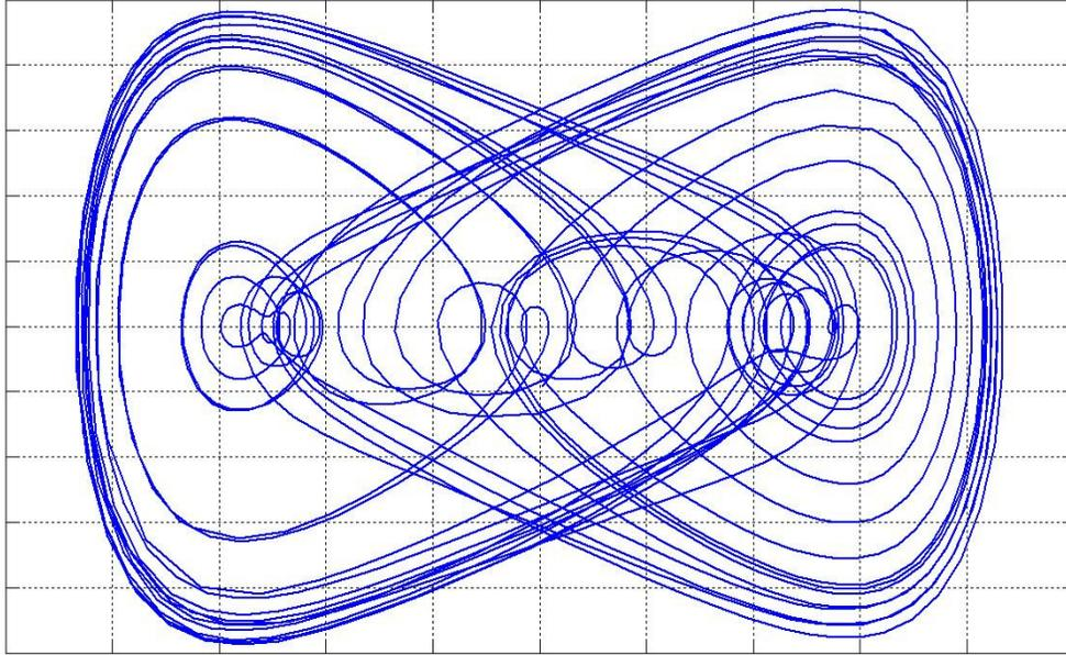
Fig. 4.3.4 - A chaotic attractor for a second-order, time-varying nonlinear system.
