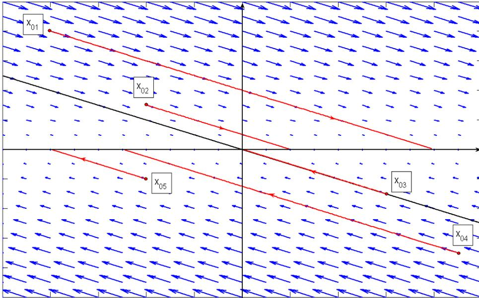
Fig. 4.1.11 - Vector field diagram for distinct real eigenvalues: one null, the other negative.
